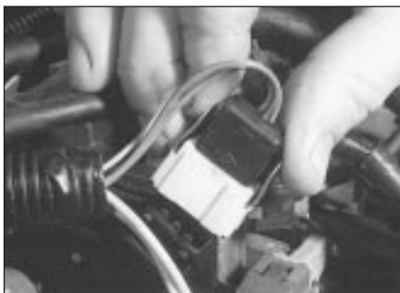
12.2a Disconnect wiring connectors from throttle potentiometer . . .
